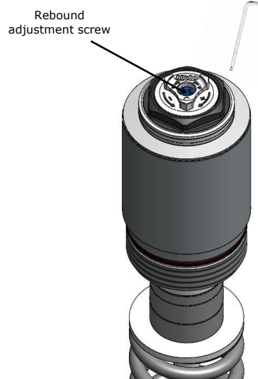
Right fork leg With Rebound adjustment
